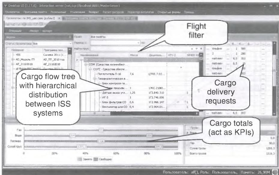
Fig. 3. Cargo flow delivery plan
