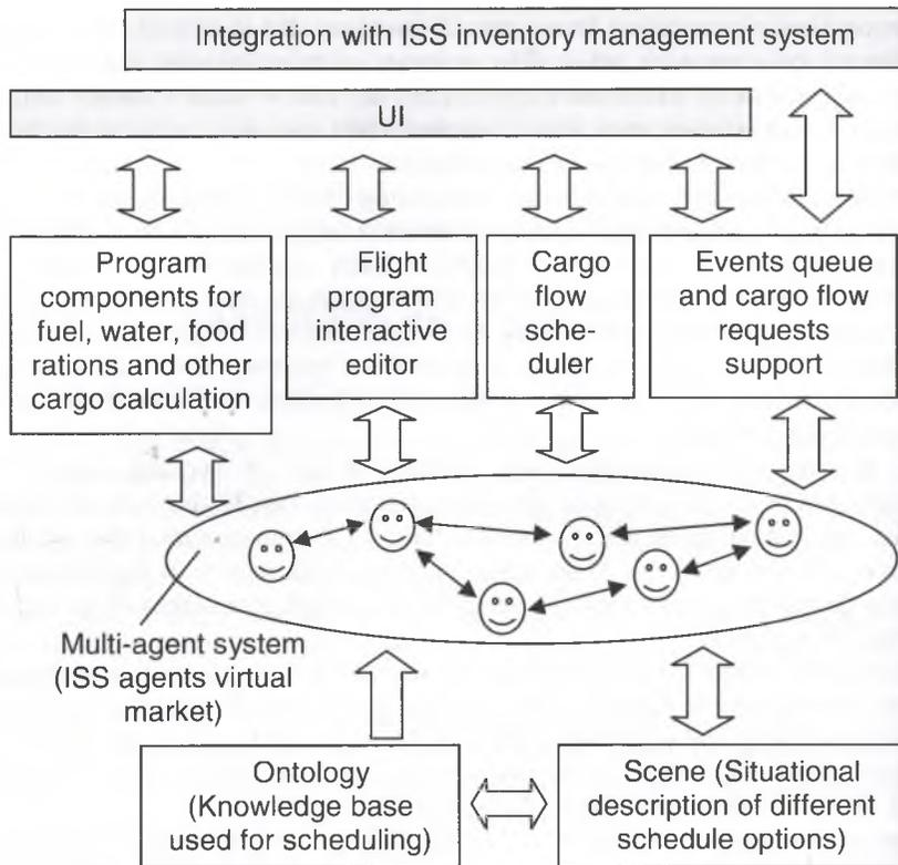
Fig. 1. Flight program and cargo flow scheduling multi-agent system architecture
